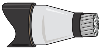
PENCILING INSULATION ON TRANSMISSION CABLE
