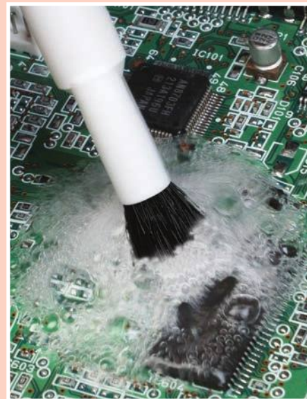
BrushClean™ System for difficult fluxes
