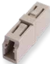
F1-8000A Multimode-Beige (No Flange) LC - Style 5 Polymer Housing Phos. Bronze Sleeve $1.50
