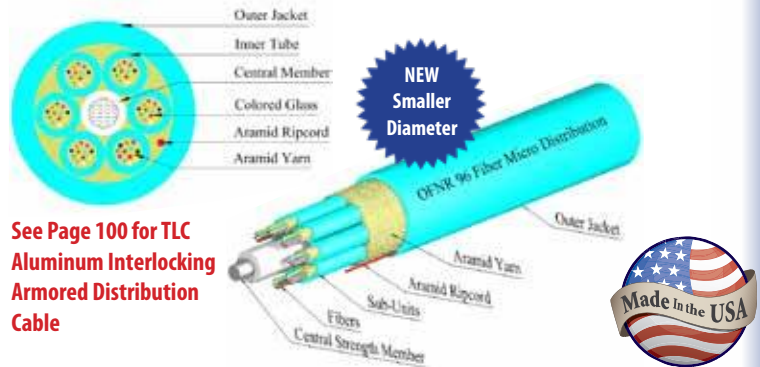
Micro Distribution Cable - 250µm Fibers
