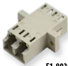
F1-8030 Duplex Multimode-Beige LC - Style 3 SC Footprint Polymer Housing Phos. Bronze Sleeve $3.25
