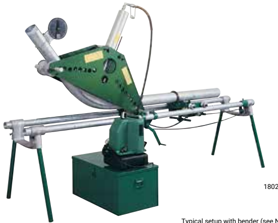
Typical setup with bender (see NOTE) Shown with 884 Bender and 980 Pump Bender and conduit not included for 1802.
