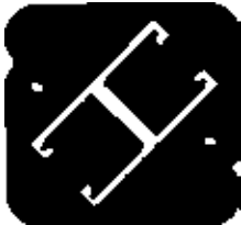
158DSTRT Back to Back Strut 1-5/8" x 3-1/4"
