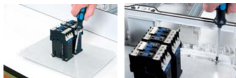
Device installation on mounting plates
