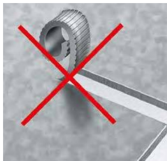
Notching without chip breaking
