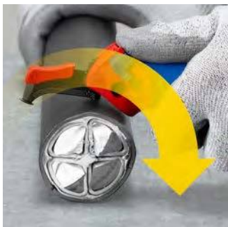
Third blade segment for round cutting
