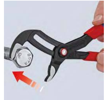
Position jaw – simply slide and close pliers
