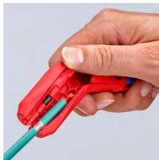
Stripping of a data cable
