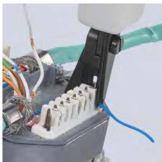
Inserts and cuts cables in one operation
