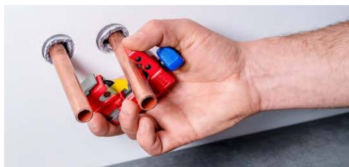
Push to the right size on the tube – or preset with the scale and click onto the tube with the spring-loaded cutting wheel
