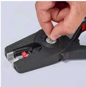
For special requirements, such as particularly hard or soft insulation materials, fine adjustments can be made using the adjusting wheel with its tactile locking positions
