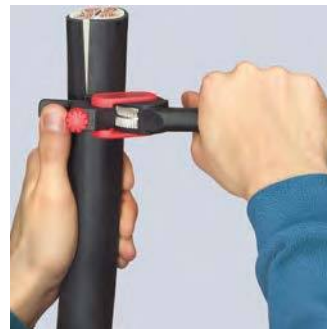
Turning the tool for circumferential cut
