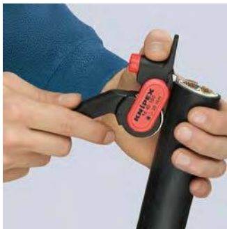
Setting the tool for longitudinal cut
