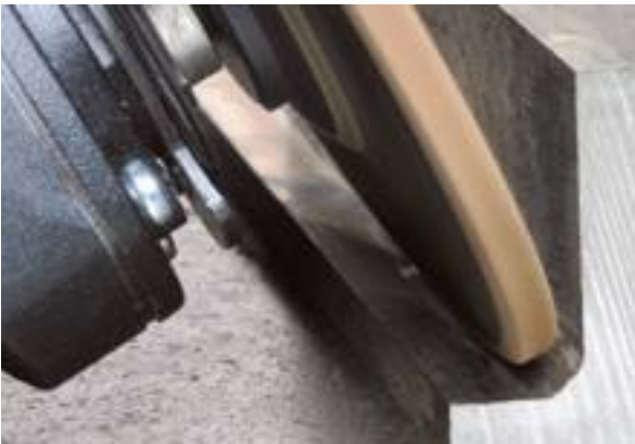
Lifetime of a grinding disc. The fine surface finish of a flap disc.
