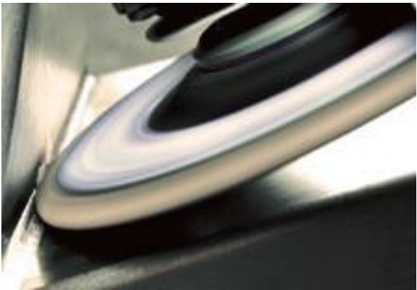
Cost-effective, as entire disc can be used for fillet weld treatment
