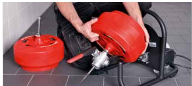
Interchangeable drum for different working ranges
