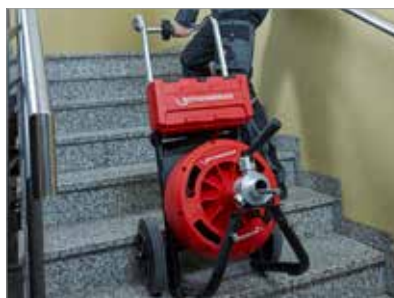
Easy transport due to stair capable chassis
