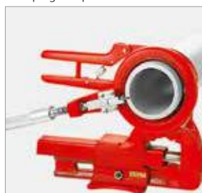
Clamping in a parallel vice
