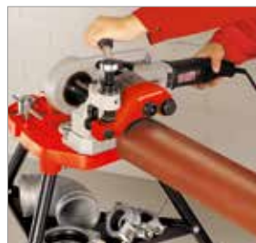
Use with roll grooving tool ROGROOVER
