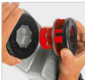
Easy insertion of the die heads
