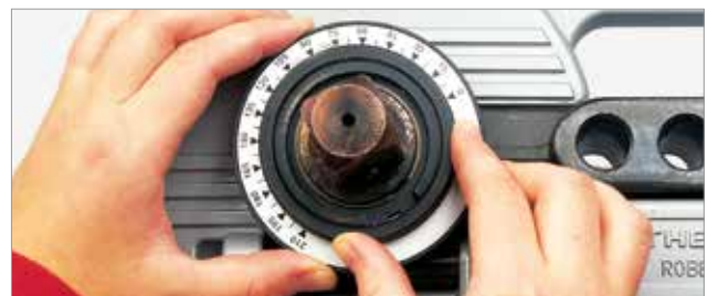
Pre-adjustment of the bending angle without tools
