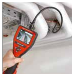
Inspection of hollow spaces
