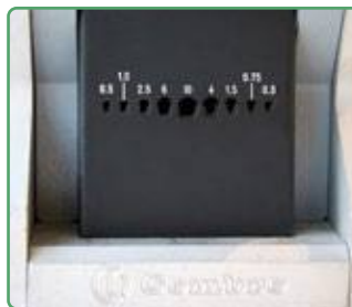
PNB-4KE detail of the crimping zone.
