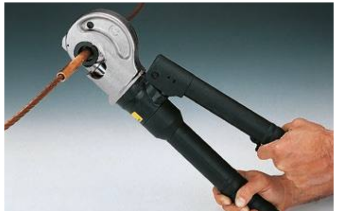
Die release system, protected from accidental operation
