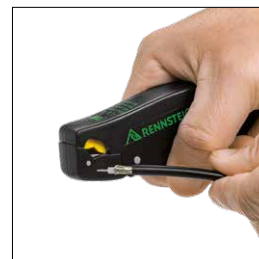
Stripping of 3 layers in one work step
