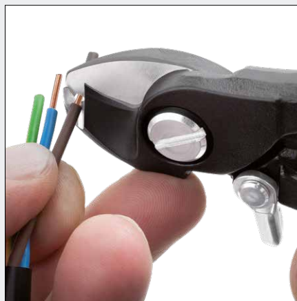
Stripping NYM/NM-B wire (1.5mm 2 – 2.5mm 2 )
