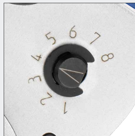
Selector position can be read off from either side of the tool
