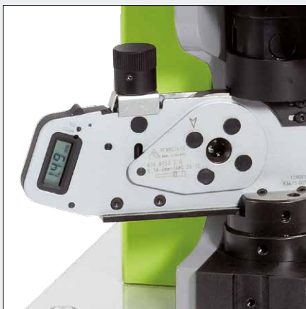
4/8 indent crimping unit with digital display
