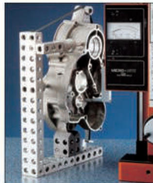
Fixtures for height gauges can be rotated by 90° allowing 2 coordinates to be measured.
