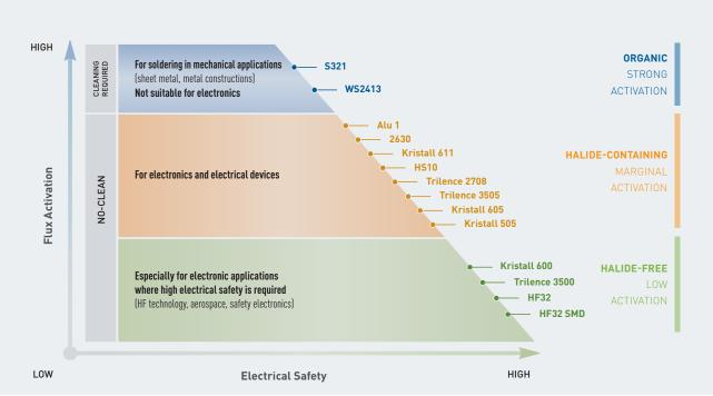
This illustration shows the relation of the flux activation to the electrical safety of the flux residues after the soldering process. For example, good electrical safety can be achieved with Kristall 611 containing an activated flux – as a No-Clean flux even without cleaning after the soldering process.
