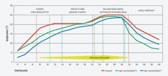
Recommended temperature profile for solder paste series in TSC305 (Sn96.5Ag3.0Cu0.5)
