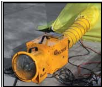
1690D & 1325D heater blower combo heating tent
