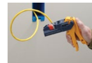
5. Pull trigger completely and remove excess wire prior to releasing trigger.
