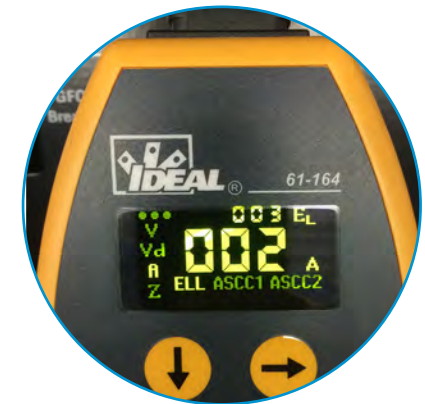
Estimated Load on Line in Amps
