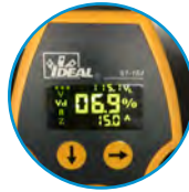
Displays Voltage Drop at 12, 15 & 20 Amps
