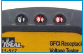
Red Lights Indicate Incorrect Wiring
