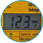
Digital Voltage Readout Provides Voltage Level at Outlet
