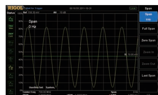
Zero span to demodulate the AM signal
