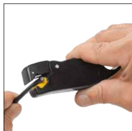
Inserting a coax cable
