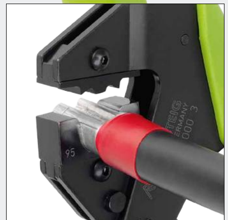
Crimping tool with 16 mm system size for processing larger wire-end ferrules
