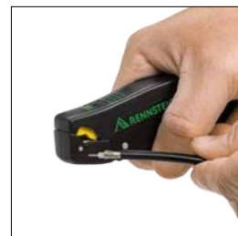
Stripping of 3 layers in one work step
