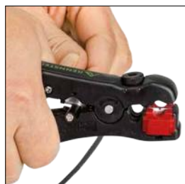
Trimming coax cables
