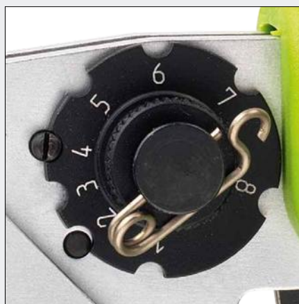
Crimp indent adjustment by 8-position selector
