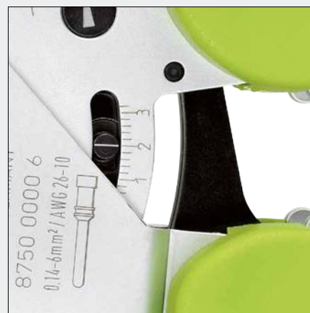
Display area, forced-lock completion of crimping process
