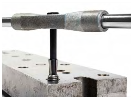
Spannen des Schraubenausdrehers mittels Windeisen Setting the extractor with a tap wrench
