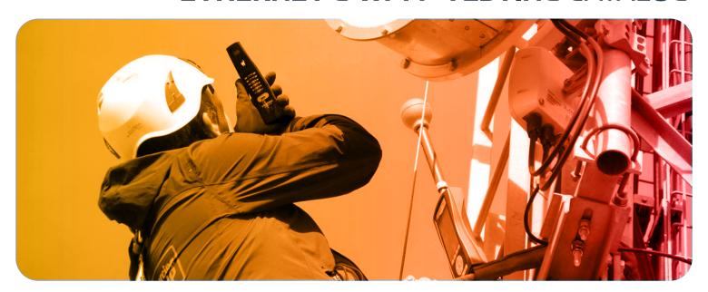
The **WaveMon RF-8** is an RF Personal Monitor for the continuous monitoring of workers' exposure to EMF. It monitors E-field up to 8 GHz and H-field up to 1 GHz. Applications include: worker's safety, telecommunications, energy, railway, medical, labs, aeronautical, industry, defense.
