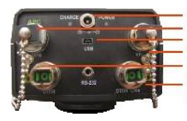
DC ChargerPort Optical Power Meter USB Port Visual Fault Locator **CHOR Port**
