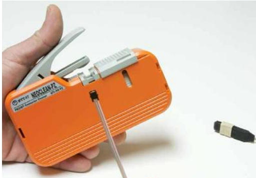
Placing PRIZM® LightTurn® connector into cleaner
