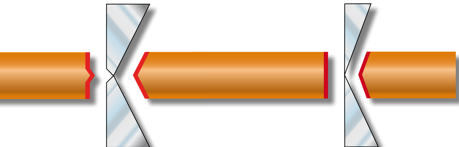
THE FLUSH CUT
