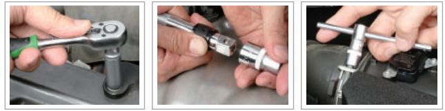
Teeth reverse flat ratchet handle Extension bar with quick release Spinner T handle
