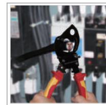
Ratchet drive for easier cutting
