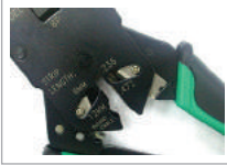
Stripping twisted pair round cable
