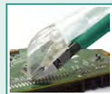
For cutting and control IC pin ends
