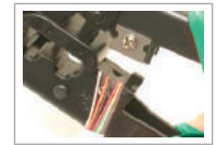
Strips flat telephone wire
