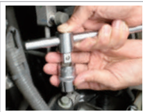
Sliding T handle with quick release
