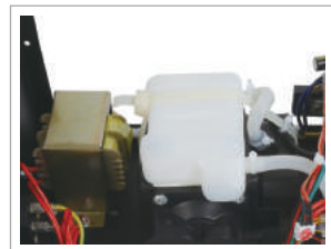
Big Air Volume Diaphragm pump produces uniform air.
