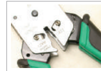
Round cable stripping
