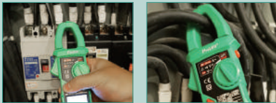
Non contact ACV detector ACA measurement
