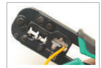
Strips twisted pair wire
