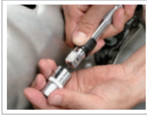
Extension bar with quick release
