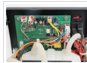
All in 1 PCB Metal screws fixed.
