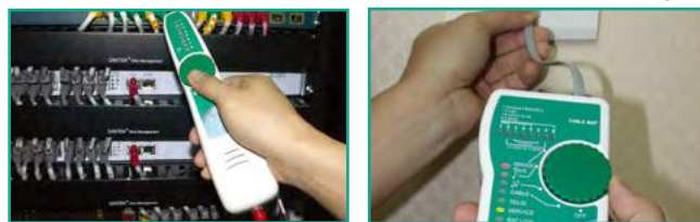
Copper cabling detecting, including shielded (STP) and UTP cable
